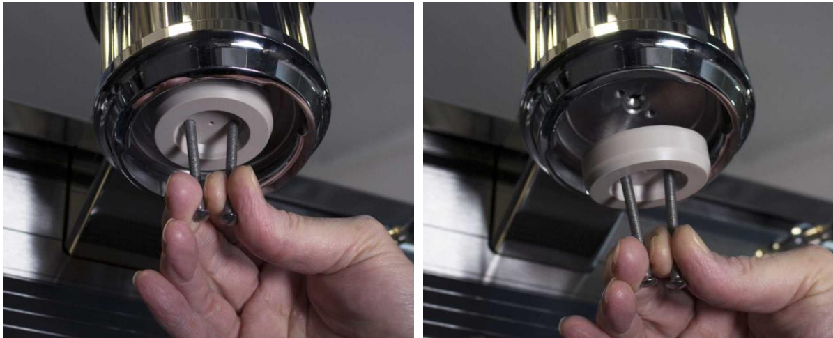
Figure 19. How to remove the dispersion base if it does not come out easily. Use 2 bolts M5x60 or similar to get grip onto the dispersion base.
