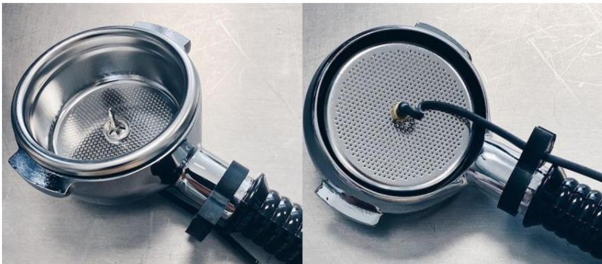
Figure 12. Temperature sensor in filter basket (mounted in bottomless portafilter).
