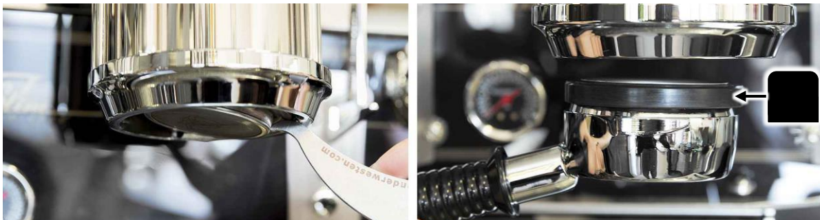
Figure 17 a (left). Pry left and right with screen extractor to remove group screen and group seal.
