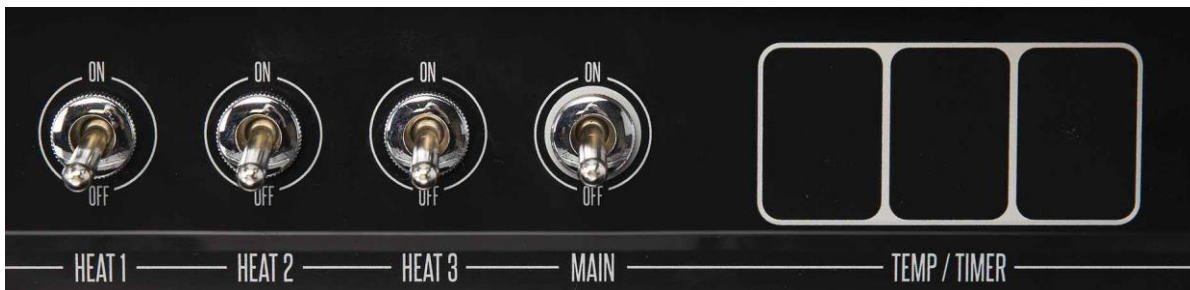
Figure 3. Showing the three HEAT switches, the MAIN switch and a blank TEMP/TIMER (3-digit) display.
