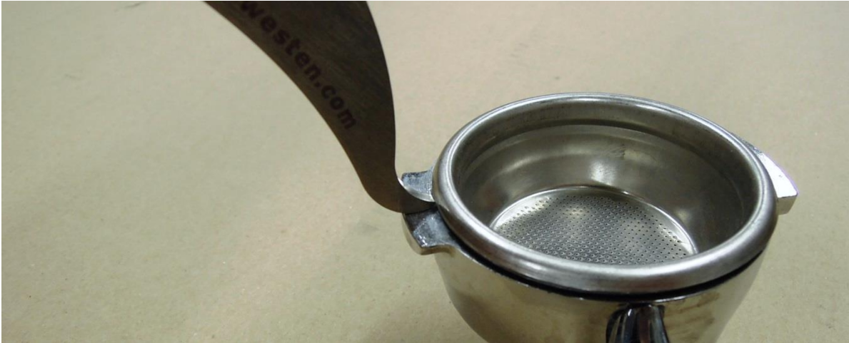
Figure 16. Pry filter basket from filter holder with the group screen extractor.
